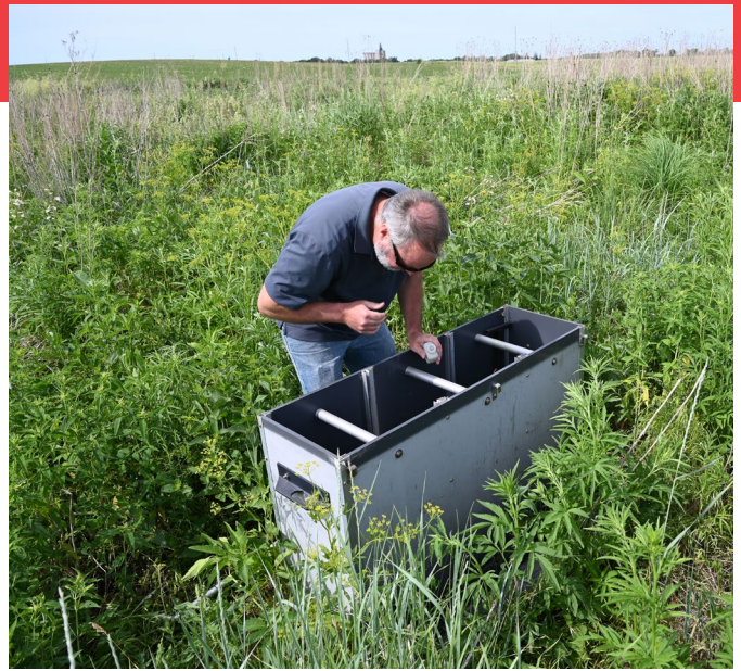
ACWA water monitoring technician Anthony Seeman pulls water samples from an established bioreactor to test nitrate-N levels from the tile-drained water entering the bioreactor.
